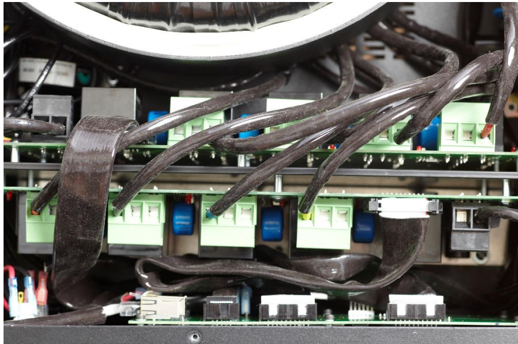
Multiple input taps on the Torus Power WM AVR 60 BAL transformer provide stable output voltage to connected equipment.
