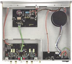
Most phono stages come in small cases so there's space to spare in the Parasound's big chassis, but this lessens hum induction, as does the screened mains transformer of the linear power supply.
